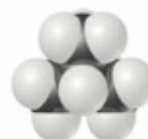
CH 3 -CH(CH 3 )-CH 3 Isobutane (2-methylpropane) mp -145° C bp -10° C
